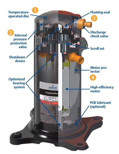
Copeland Scroll compressors feature a variety of internal safety controls, designed to ensure proper actuation of the internal line-break motor protection. These safety features include:
