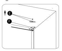
3. Remove the upper hinge (Please hold upper door by hand when installing). Keep it for future use.
