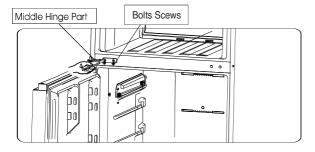
13. Hold the freezer door in the appropriate position. Make sure the door is level and insert the middle hinge axis into the into the lower hole of the freezer door.
