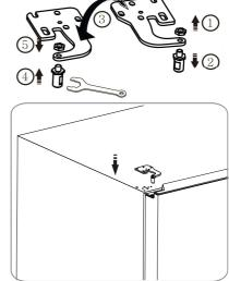
15. Remove the upper hinge cover from the plastic bag provided, and install it and fix it with screws.
