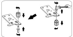
10. Move the lower hinge part to the left side and screw it on with the special flange self-tapping screws. Move the adjustable bottom feet parts to the other side and screw them.
