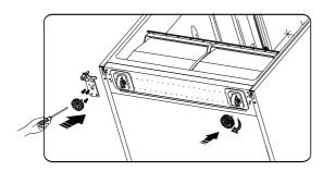
11. Stand the refrigerator upright and carefully slot the fridge door onto the lower hinge pin and hold it in position.
