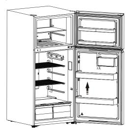
2. With the door closed, remove screws (you can pry it up with a Philips Screwdriver) and the upper hinge cover (you can pry it up with a Slotted Screw driver) (E) on the top right side of appliance and remove 3 special flange screws (F) with a Socket Wrench. Keep the upper hinge cover for future reference.
