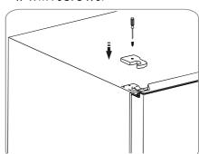
16. During reversing the door, you can adjust the upper hinge to make the door seal flat against the refridgerator. Don't leave any gaps.
