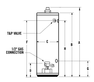
Maximum Hydrostatic Working Pressure: 150 PSI
