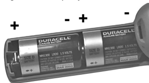
Figure 1. Properly Installed Alkaline Batteries
